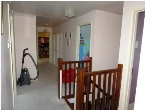
The walls and ceilings are plastered finished with emulsion with no significant cracking noted.
